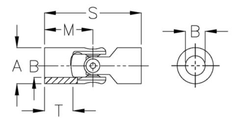
$\begin{array}{lll} A & = 20 \\ B \ H7 & = 10 \\ M & = 24.0 \\ MD \ max \ N \ m = 15 \\ s & = 48 \\ T & = 13 \end{array}$
